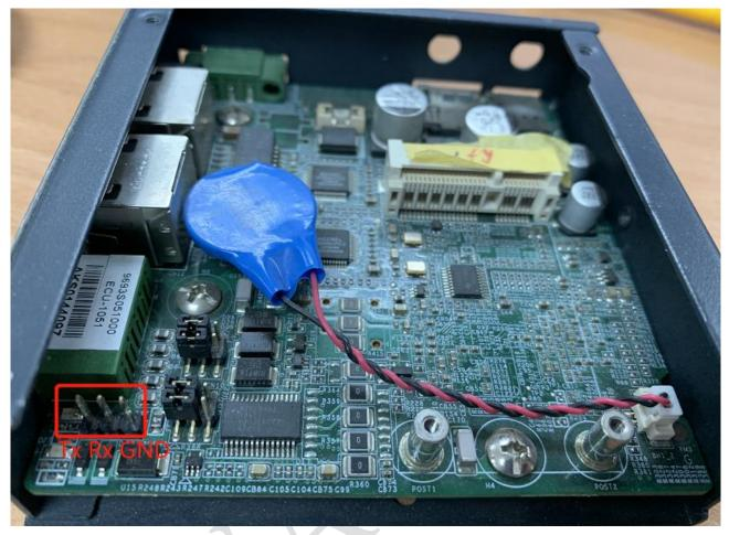
CN8 inside the ECU-1051. The picture above shows the ECU pins Note: the console is not the COM1/2 outside.
